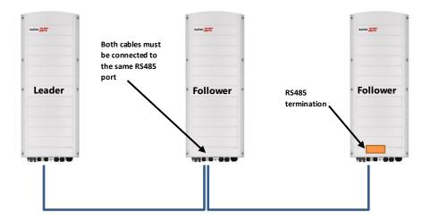
RS485 is a bus connection, which means the wires must be connected from one inverter to the other (starting from the leader); the middle inverters must have 2 cables connected in parallel. Refer to the product installation manual for detailed instructions on leader/follower inverter connections.
