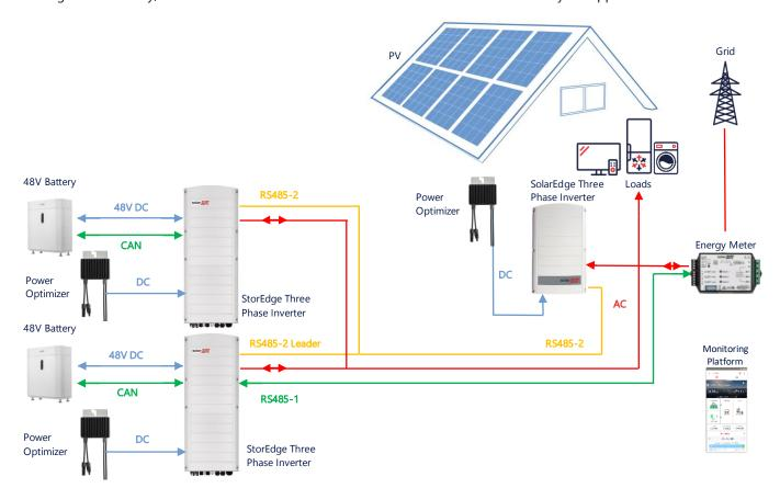
Up to three StorEdge Inverters can also have Power Optimizers or can be AC-Coupled to a non-SolarEdge power source, as explained in the below use case. In case three Home Hub inverters are used with other three phase inverter from SolarEdge, the other inverter CANNOT be connected to the leader as a follower. In other words, no more than 3 inverters can be connected on a leader-follower configuration.
