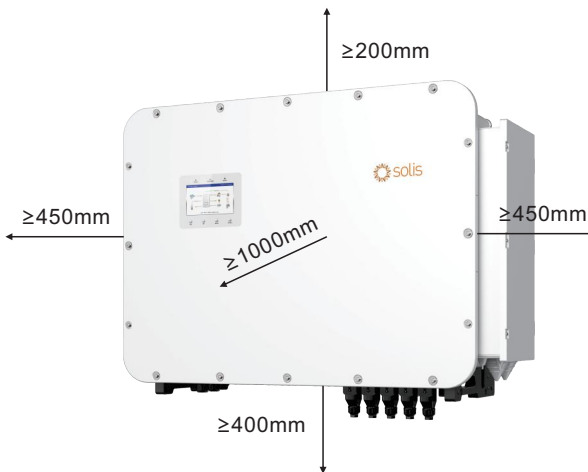
Figure 3.3 Inverter Mounting Clearances
