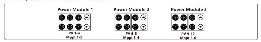
9 string equally powered design will not effect your maximum production. On different oriented strings such as west and east, for best power generation it should be distributed to each power modules as proportional. 88kW is divided to 3 modules for 29.33kW max production in each module. Our recommendation is a power balance of the modules for best performance.
