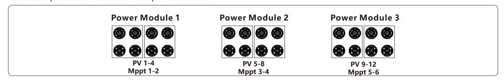
12 string equally powered design will not effect your maximum production. On different oriented strings such as west and east, for best power generation it should be distributed to each power modules as proportional. 88kW is divided to 3 modules for 29.33kW max production in each module. Our recommendation is a power balance of the modules for best performance.
