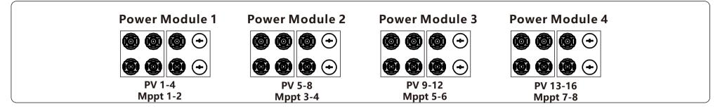
12 string equally powered design will not effect your maximum production. On different oriented strings such as west and east, for best power generation it should be distributed to each power modules as proportional. 121kW is divided to 4 modules for 30.25kW max production in each module. Our recommendation is a power balance of the modules for best performance.
