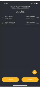
10. Once you have entered all the devices, you can change the priority of the devices by holding and sliding the three horizontal lines on the far right. A high priority means that this device is preferred when surplus solar power is scarce.
