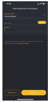
6.Select the inverter that is installed at your customer's site from the list (via "Device name"). When you prepare the installation leave the field for the IP empty. You can find information about other settings such as "Device ID" under the yellow link "Solar Manager" directly below the settings. Click on "Save".
