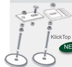
Special fixation on sheet metal roofs FixPlan
