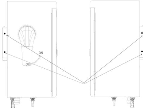
Screw from right side of wall mounting bracket
