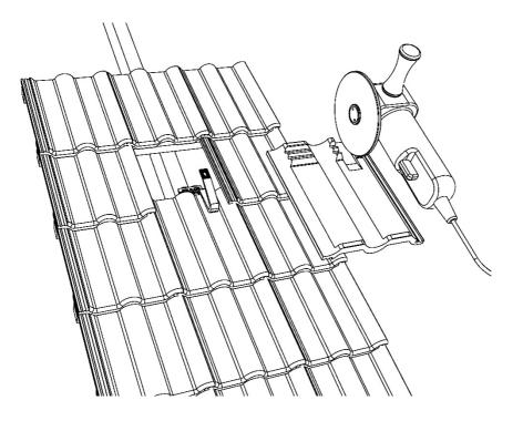
Remove the bar so that there is at least 5 mm clearance around the roof hook in the next step!
