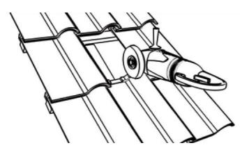
Only remove the raised edge; never ablate any deeper. Only remove the raised edge to the extent that the minimum distance is maintained.
