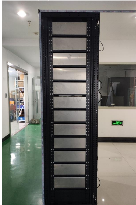
Figure 8 Battery System (Side view for 25 modules)
