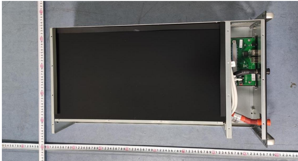
Figure 13 Battery pack (Remove top cover)
