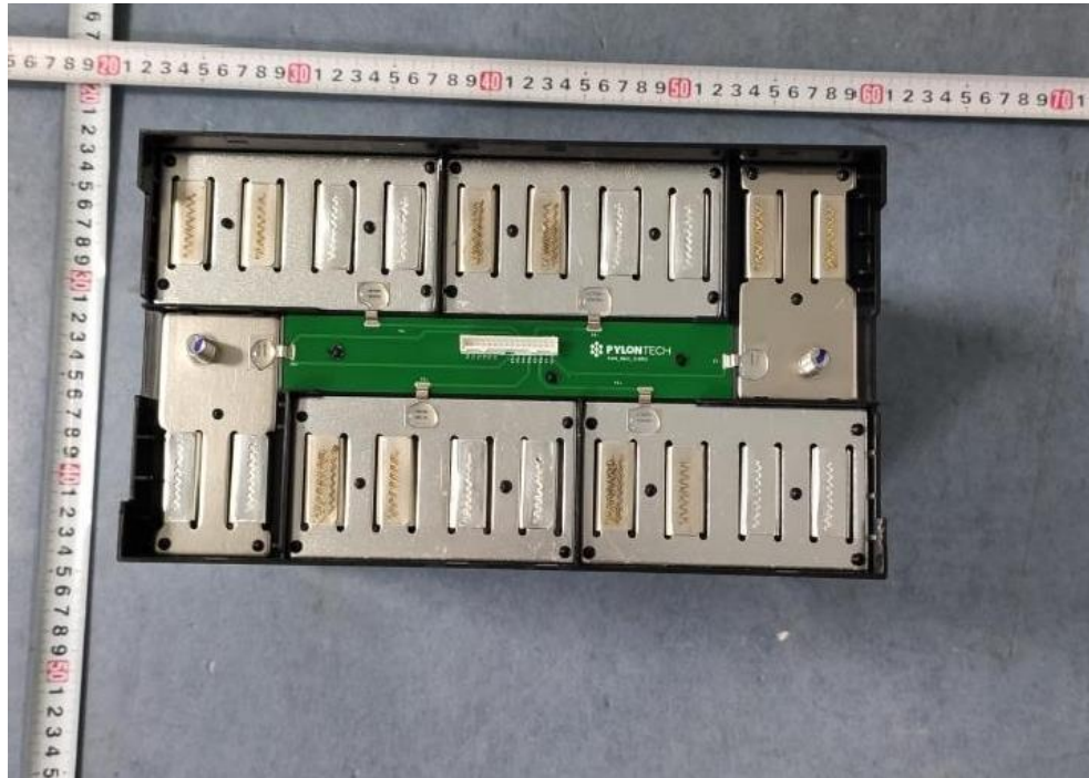
Figure 21 Module (Terminal view inside pack)
