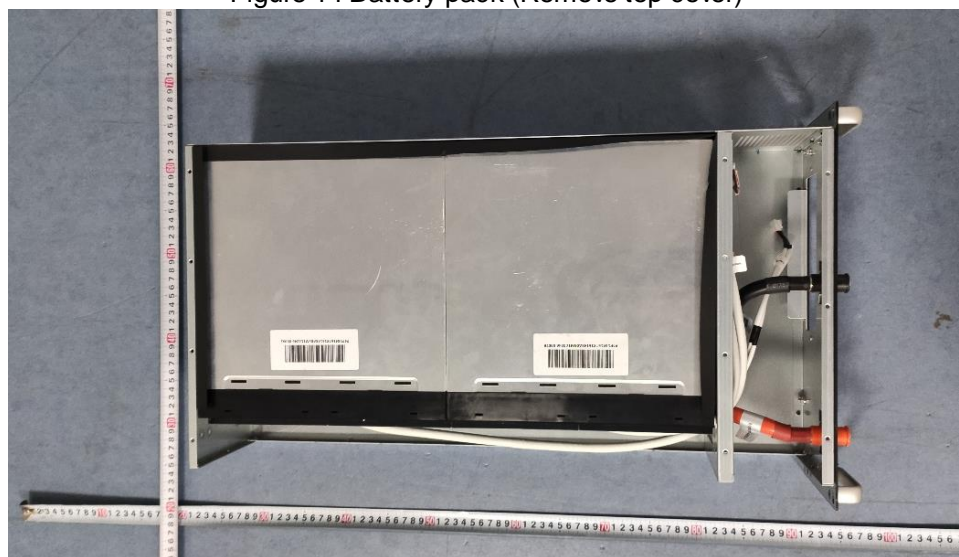
Figure 15 Battery pack (Remove top cover)
