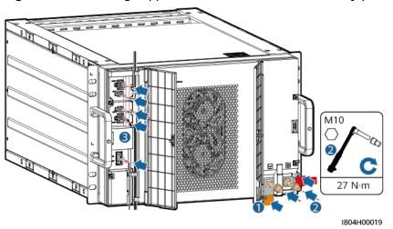
**Figure 4-32** Installing copper bars and cables for the battery pack
