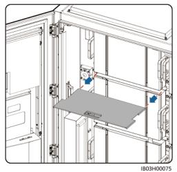
Figure 4-29 Removing the protective plate
