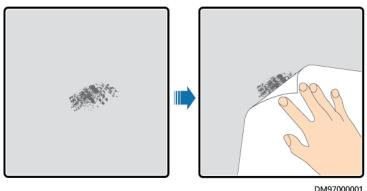
**Step 2** Dip a piece of cotton cloth into anhydrous alcohol and wipe the polished or damaged area to remove the dirt and dust. Then wipe off the anhydrous alcohol with a clean and dry cotton cloth
