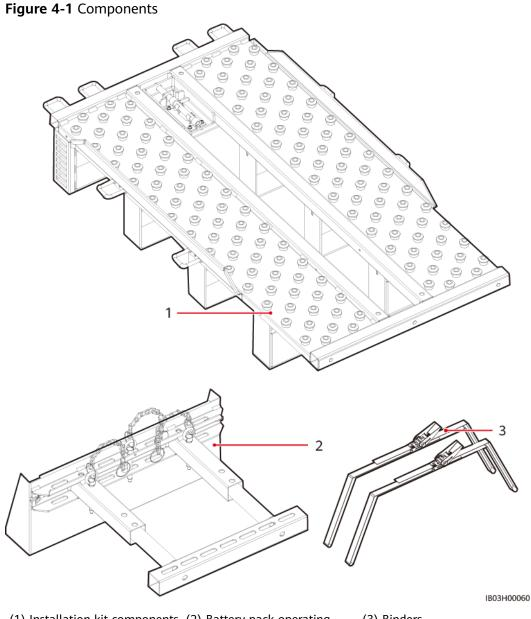
(1) Installation kit components (2) Battery pack operating (3) Binders handle
