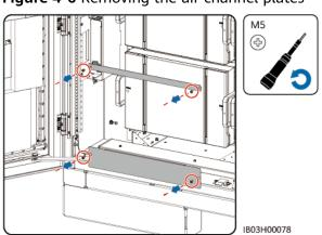
Figure 4-6 Removing the air channel plates
