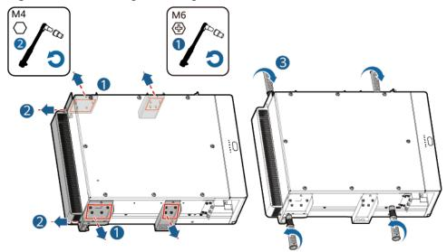
Figure 8-10 Removing mounting kits
