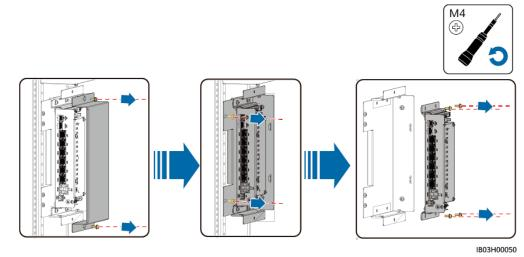
Figure 27-2 Removing the I/O expansion board
