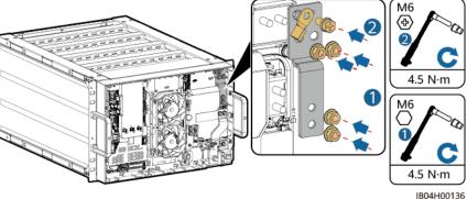
Remove the insulation tape from the flat cables and install the flat cables to the Step 9 management module.
