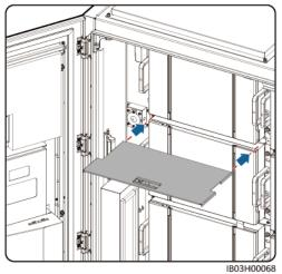
Figure 4-21 Installing the protective plate
