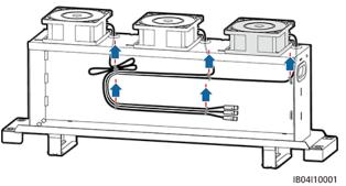
Figure 9-4 Removing the FAN 1 cable ties
