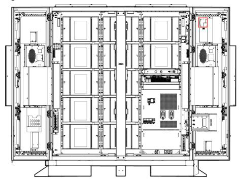
Figure 24-1 Position of the exhaust fan
