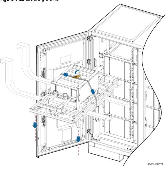
**Step 16** Remove the positioning pin, binding straps, and shovel pan.
