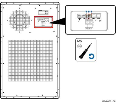
Figure 10-11 Removing air conditioner cables
