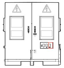
Figure 15-1 Position of the emergency stop switch
