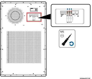
Figure 10-2 Removing air conditioner cables
