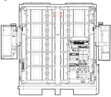
Figure 19-1 Positions of door status sensors
