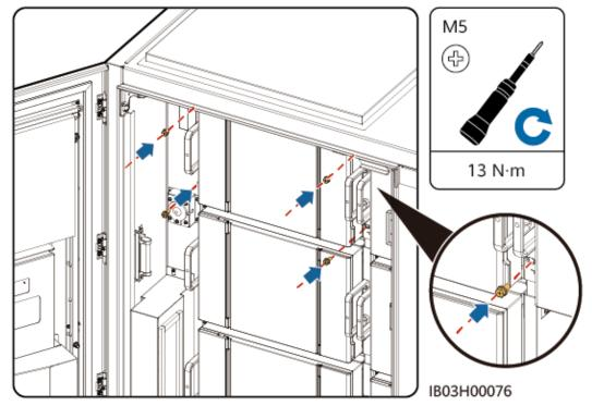
**Step 12** Install air channel plates between battery packs based on the label on the air channel plates. The air channel plates are delivered with the product.
