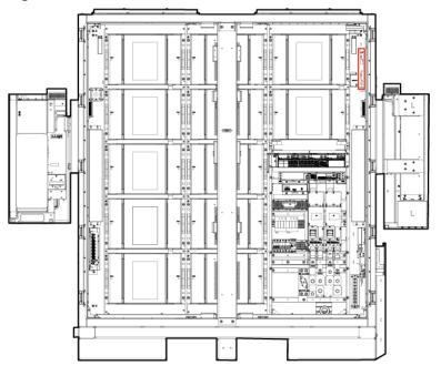
Figure 22-1 Position of the exhaust controller (TCUE)
