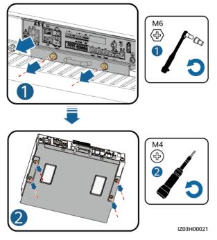
**Step 3** Remove the mounting ears and guide rail-mounting brackets from a new CMU, and install the cabinet-mounting bracket.
