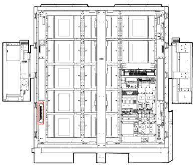
Figure 27-1 Position of the I/O expansion board
