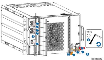
Figure 4-4 Removing copper bars and cables
