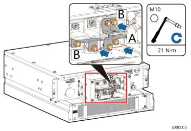
**Step 12** Install cables to the BAT/BUS, J1, and J2 terminals, and FE network cable for the rack controller.
