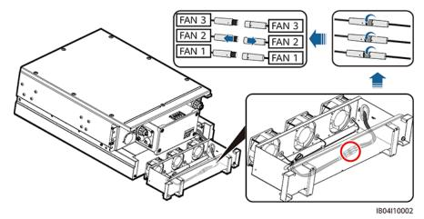
**Step 4** Remove cable ties from the faulty fan.
