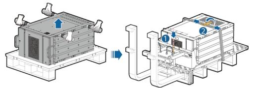
Figure 4-11 Moving the new battery onto the installation kit
