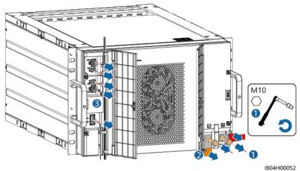
Figure 4-16 Removing copper bars and cables
