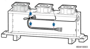
**Step 5** Remove the faulty fan (FAN 1 is used as an example).
