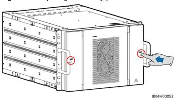
Figure 4-15 Opening the battery pack covers
