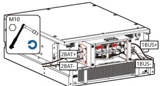
**Step 3** Remove the J1 and J2 terminals, and the FE network cable.
