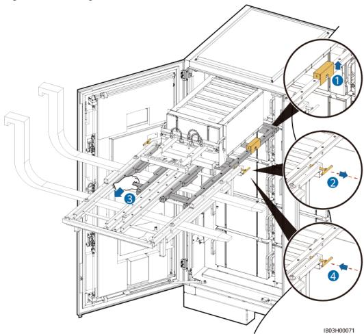
**Step 15** Install binding straps and lower the kit.
