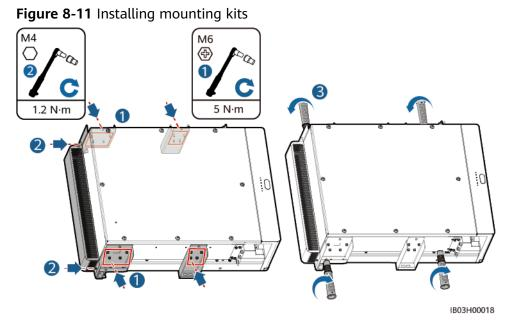
**Step 10** Install the new rack controller to the mounting bracket on the ESS.
