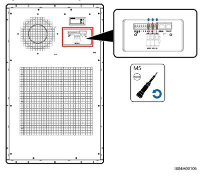
Figure 10-17 Removing air conditioner cables
