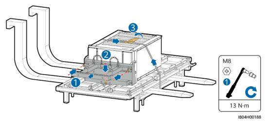
Step 4 Lift up the kit and remove the battery pack binding straps.
