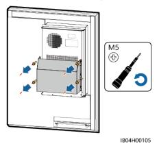
**Step 2** Remove cables from the air conditioner.
