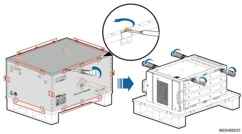
**Step 2** Move the battery pack onto the kit base, and remove the lifting handles.
