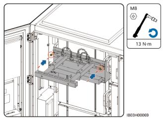
Figure 4-22 Installing the battery pack shovel pan
