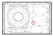
Figure 10-5 Removing the internal fan cable
