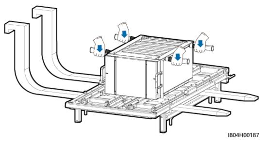
**Step 3** Install the shovel pan, positioning pin, and binding straps.
