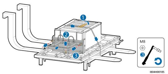
**Step 17** Install the lifting handles and remove the old battery pack.
