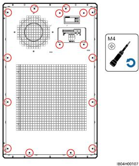
**Step 4** Remove the screws from the fixing plate of the internal fan, and then remove the internal fan and the fixing plate.
