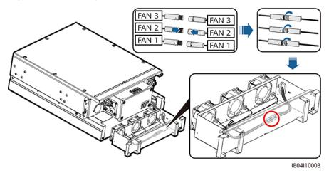
**Step 9** Push the fan tray into the slot and tighten the screw.
