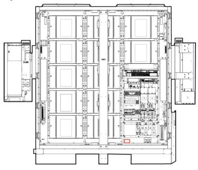
Figure 20-1 Position of the water sensor
