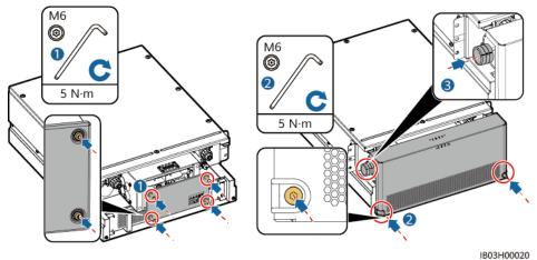
**Step 14** Install the protective covers, connect the ground cable, and bind the cable. Bind and secure the magnetic rings and the protective covers.
