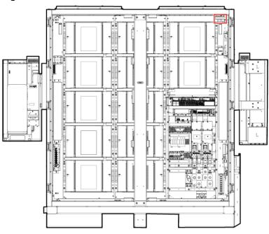
Figure 26-1 Position of the smoke detector
