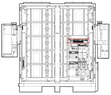
**Figure 16-1** Position of the embedded power subrack
