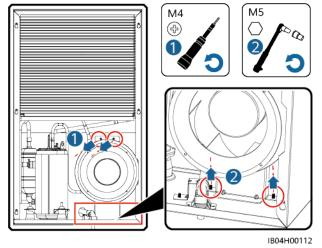
**Step 3** Remove cables from the quick connect port of the external fan, and remove the external fan from the support.
