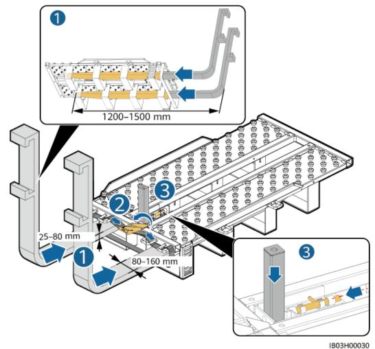
**Step 9** Install the operating handle on the battery pack, pull the old battery pack onto the installation kit, and secure the battery pack.
