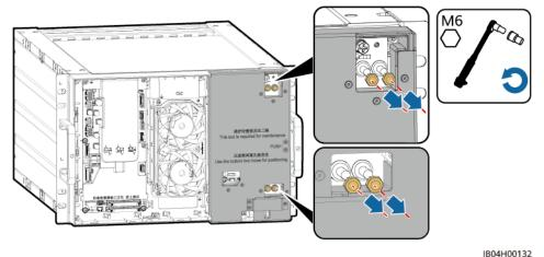
**Step 7** Remove the 10 screws from the management module and remove the management module (including the battery pack fixture).
