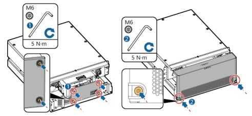
**Step 6** Remove the ground cable and the delivered protective covers.
