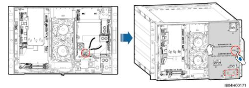
Figure 5-5 Installing the battery pack fixture
