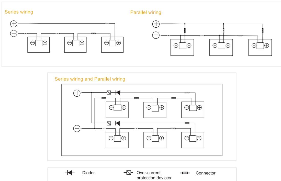
Figure 4: Electrical diagrams of series and parallel wiring
