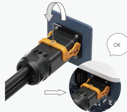
**3** Tighten the screws with the S2.5 hexagon wrench with a torque of  $2.5 \pm 0.1 \text{ Nm}$ . Installation completed.
