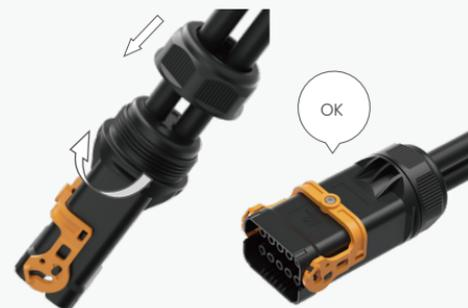
**5** Seal plugin to main body. Tighten the nut with an open-ended wrench (torque  $10.0 \pm 0.1 \text{ N}\cdot\text{m}$ , Complete the installation)
