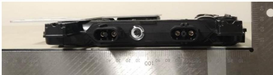
*Figure 6: IQ7PLUS Connector side*
