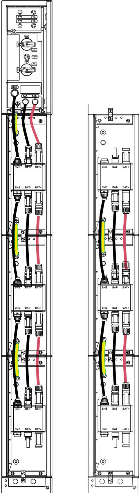
2. Connect cables between the bottom modules.
