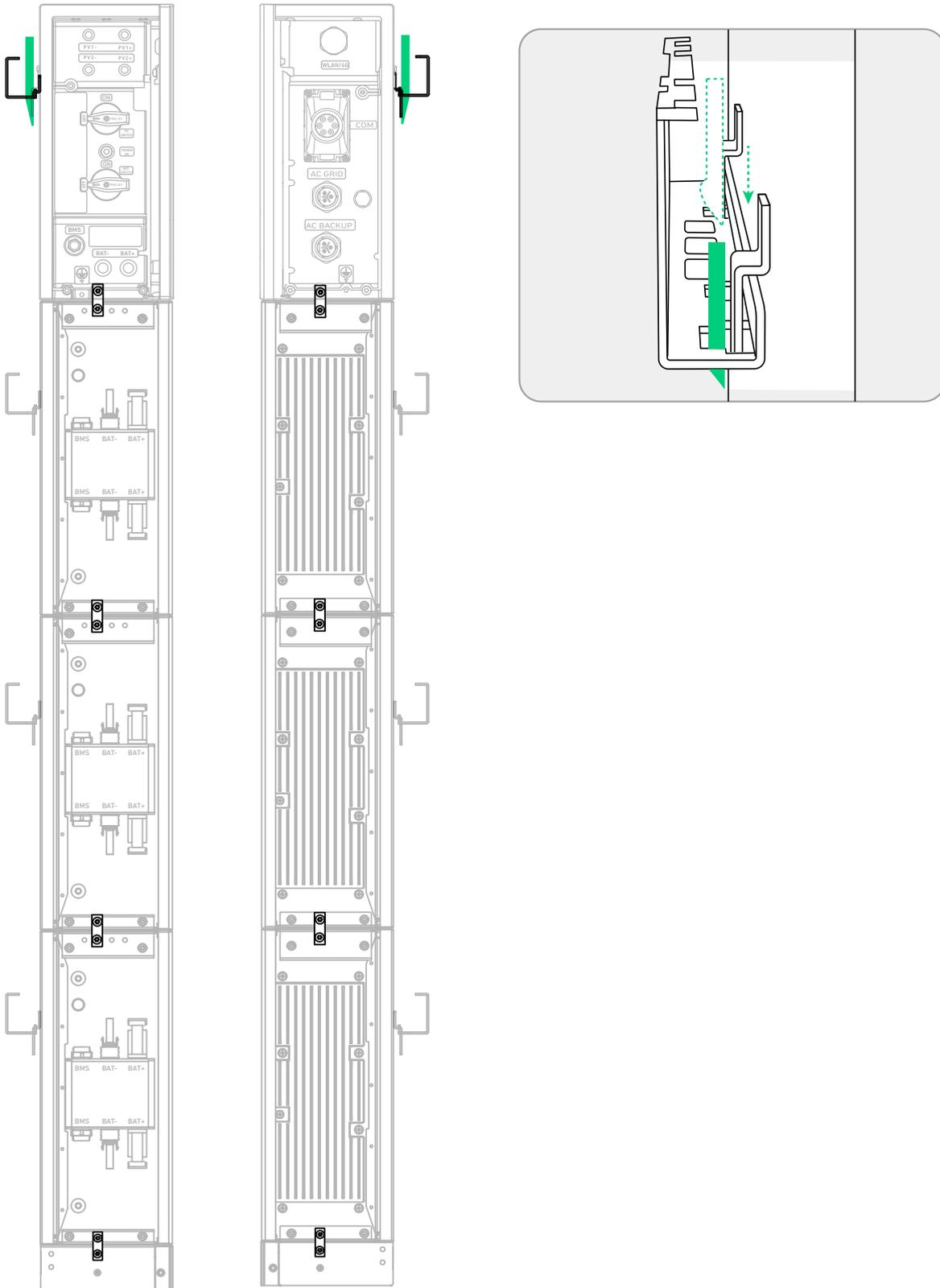
3. When adding the second column, attach the top cover to the top battery module using the screws (M5×14 mm, included).
