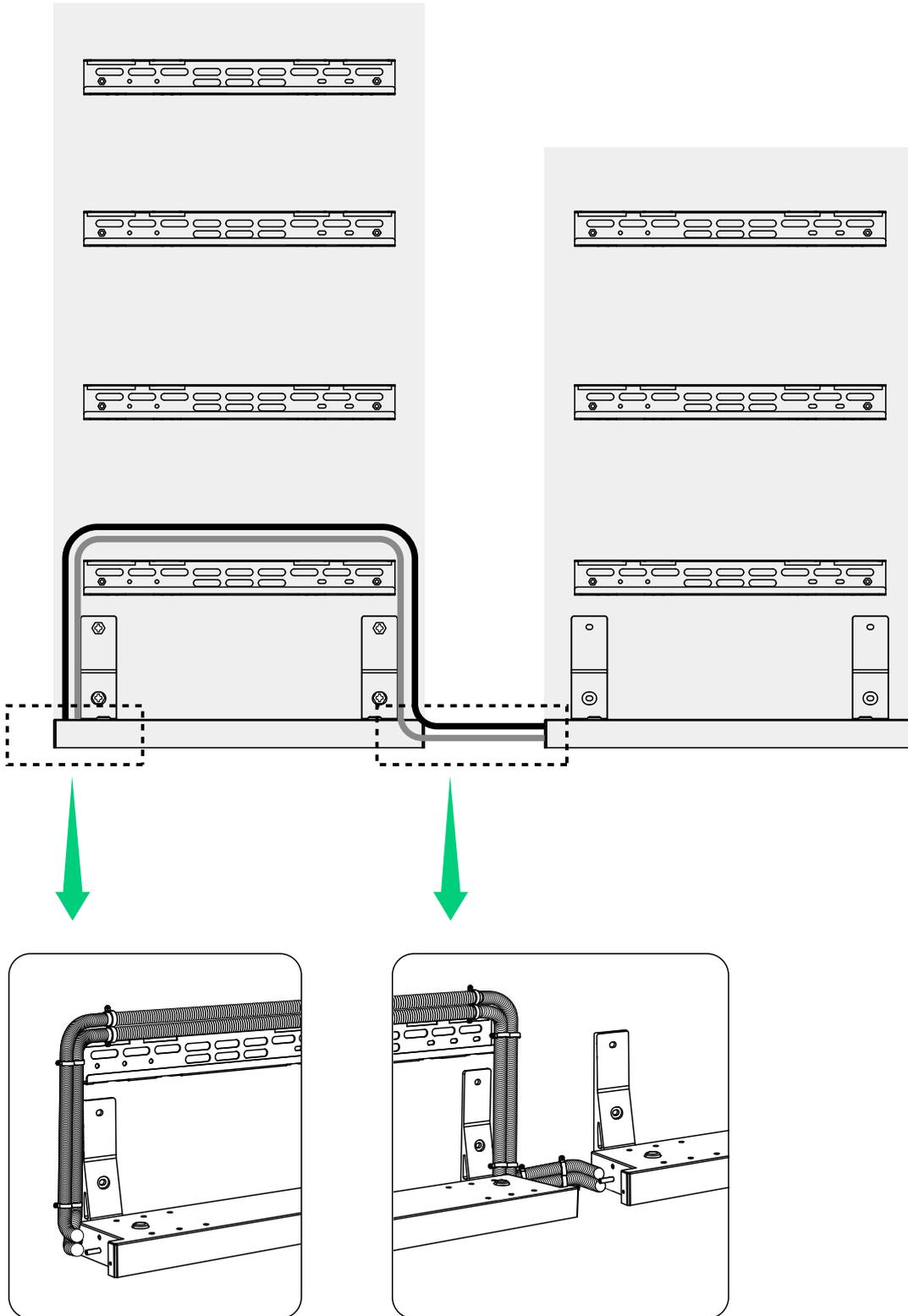
**Step 5: Mount modules onto the brackets.**
