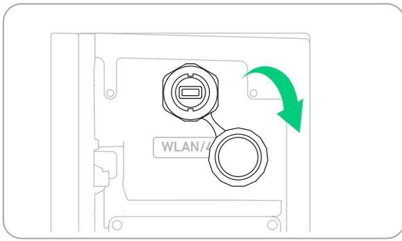
③ Install the appropriate dongle according to the networking methods.
