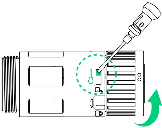
2. Route a 3-conductor AC power cable (7-12.5 mm in outer diameter, not included) through the nut and body. Then, strip the insulation layers from the conductors.
