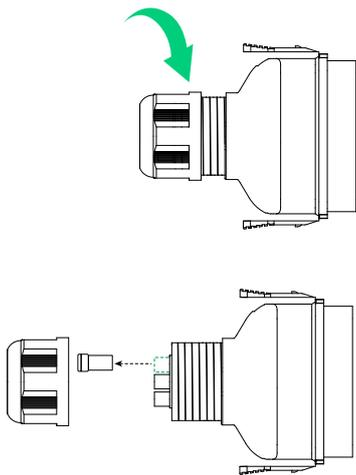
3. Route the 2-wire RS485 signal cable (5.5±0.5 mm in outer diameter, included) through the locking cap and wiring compartment cover.
