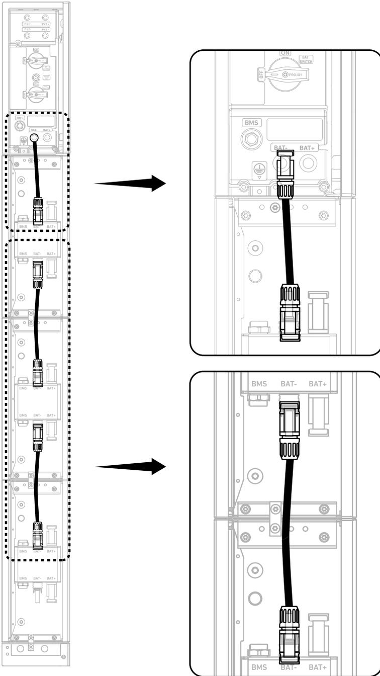
5. Connect the positive DC power cables between the modules.
