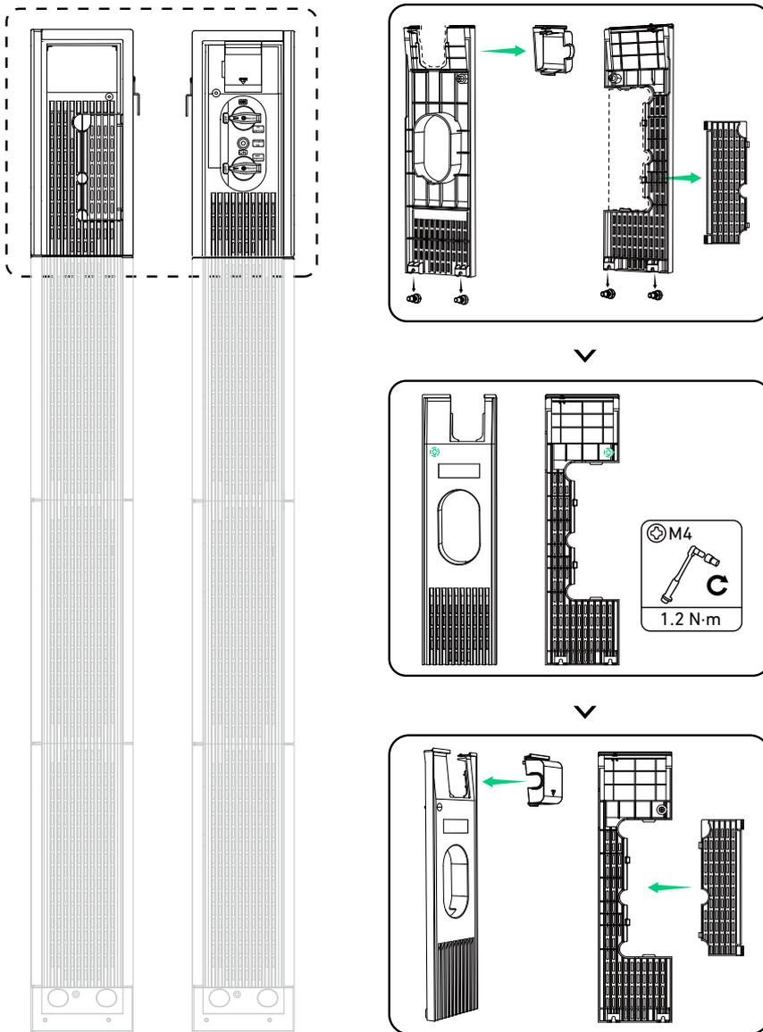
3. Attach the baffles to the modules.
