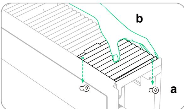
② Open the WLAN/4G port cover on the right side of the power module.
