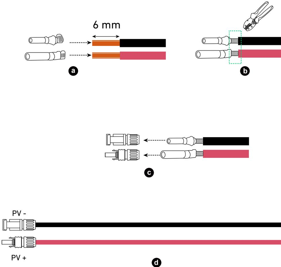
3. Connect the positive PV connector to a positive PV power port (PV1+ or PV2+) and the negative PV connector to a negative PV power port (PV1- for PV1+, or PV2- for PV2+).
