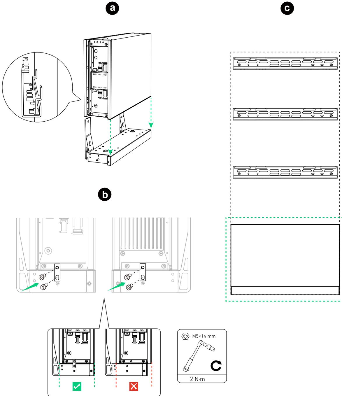
2. Mount the remaining power module and battery modules from bottom to top.
