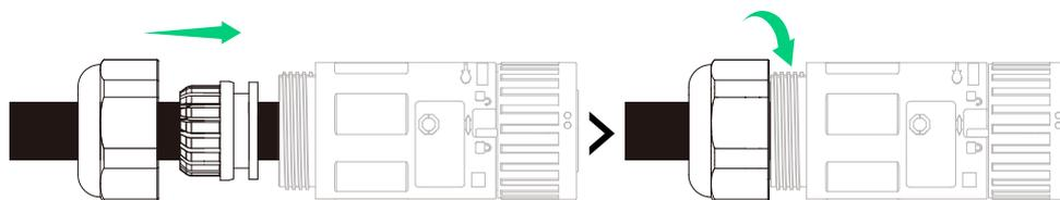
8. Repeat steps one to seven to assemble the AC backup connector (male, included).
