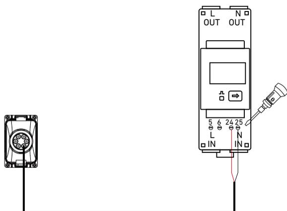
8. Connect power wires to the grid-side power sensor.
