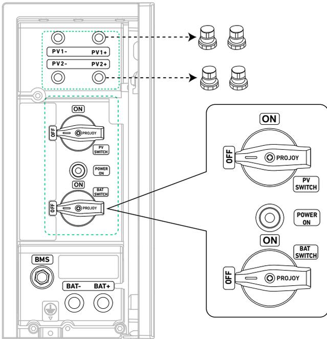
2. Strip the insulation layers on the ends of the positive and negative PV cables (not included). Crimp the positive and negative metal terminals (included) onto the corresponding cables. Make sure the terminals are securely attached and cannot be pulled out. Insert the positive and negative metal terminals into the corresponding PV connectors (included). You should hear a click when they are properly connected. Tighten the locking nuts to secure the connection.
