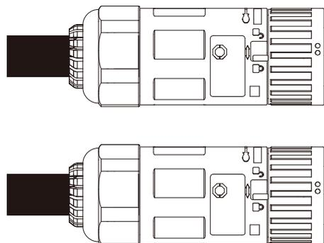
9. Remove the dustproof covers from the AC power ports. Then, insert the AC grid connector (female) to the AC grid port, and insert the AC backup connector (male) to the AC backup port. Rotate the locker in the locking direction to tighten the connectors.
