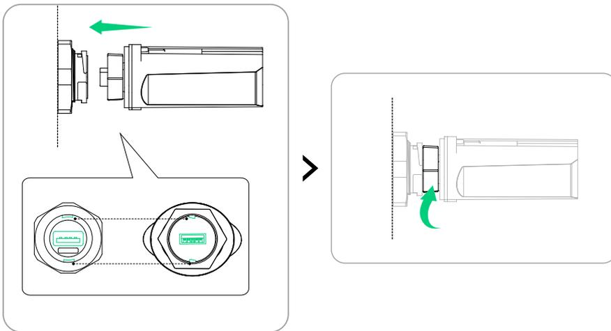
④ Press the back of the panel to reinstall it, and then tighten the screws (M3×8 mm).
