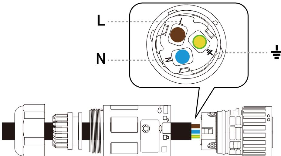
5. Tighten the three screws on the housing with a No. 1 Phillips screwdriver.
