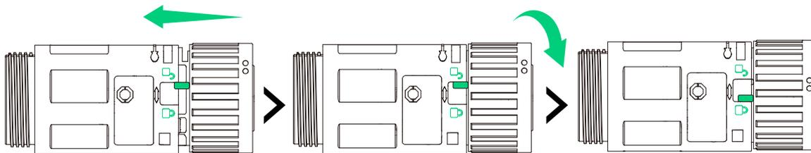
7. Tighten the nut to secure the cable.
